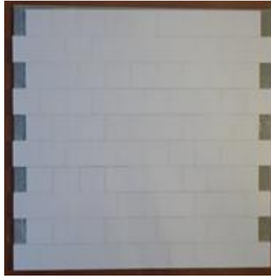
Figure 3. Alumina ceramic / glass-polyester composite panels for ballistic testing.
