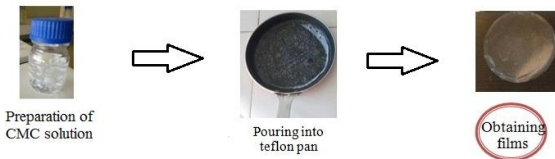
Figure 1. Preparation steps of CMC films
