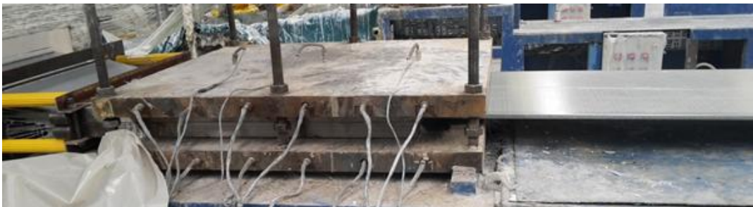
Figure 2. Image of the pultrusion process line used to produce resin based composite panels.
