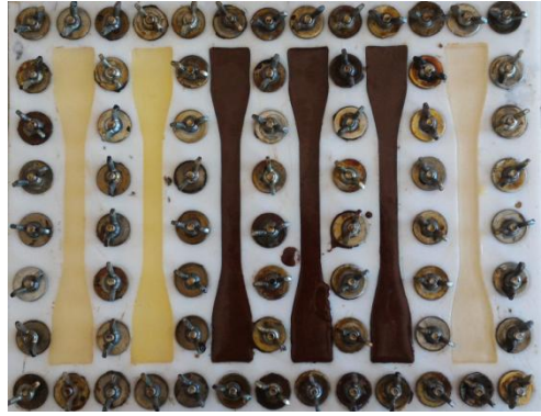
Fig. 1. Preparation of mold composites according to ASTM D 638 standards
