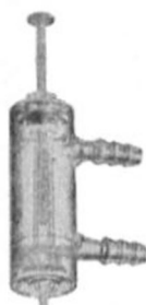
Syringe Mantle Device for keeping sample in syringe at a constant temperature.
